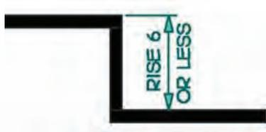
Figure 35: Changes in Level up to 6 mm
