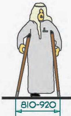
*Figure 5: Clear Floor Space for a Person using Crutches*
