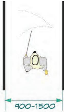
Figure 7: Clear Floor Space for a Person using a Long White Cane
