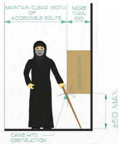
Figure 40: Limits of Protruding Objects
