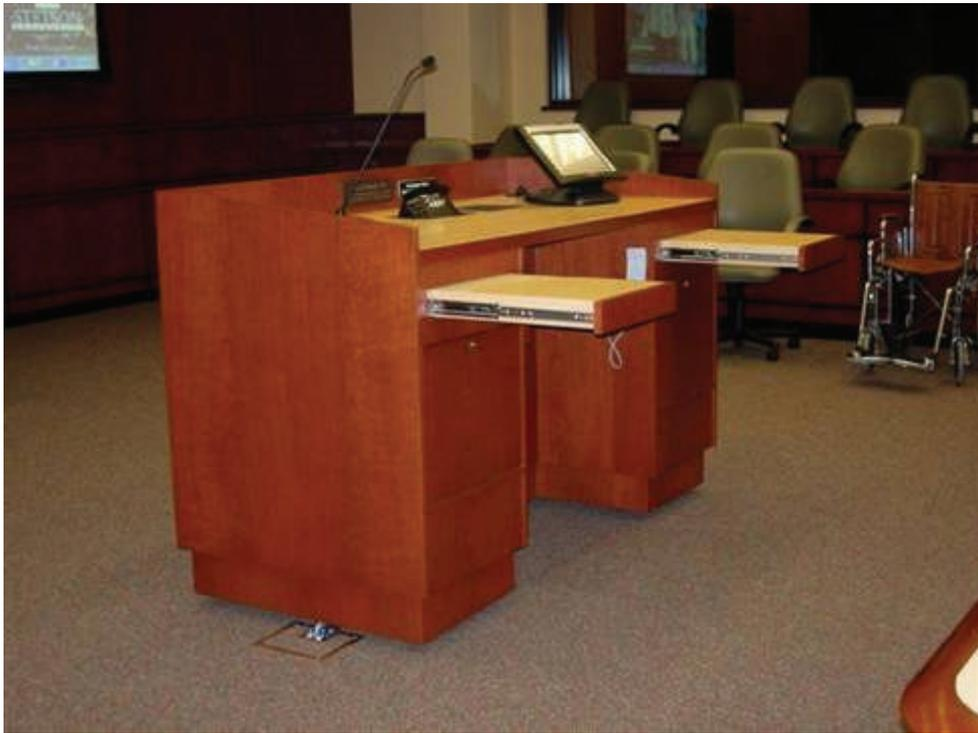
*Figure 35. Accessible lectern with knee and toe clearance*
