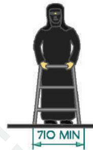
Figure 111. Clear Floor Space for a Person using a Walker
