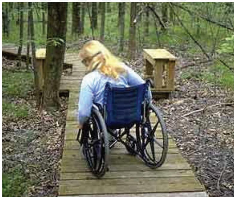
*Figure 74. The usage of raised and leveled walkways and circulation routes, with intermittent passing areas constitutes an essential service offering for parks and tourist services relying on exterior interfaces.*
